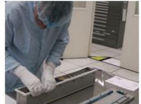
Figure 6 Final assembly of new Charcoal Filters at KSC
